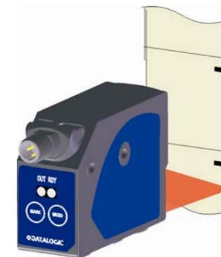
The DARK/LIGHT operating mode is automatically selected by the sensor. Dark mark - light background = dark mode; light mark - dark background = light mode.
